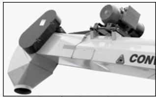
Fig 47 - Speed Reduction Drive
