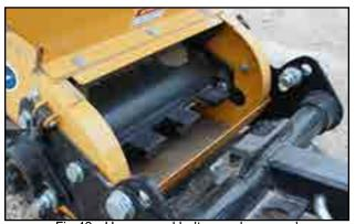
Fig 42 - Hopper end belt, guard removed
