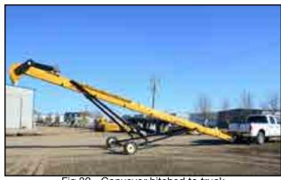
Fig 30 - Conveyor hitched to truck
