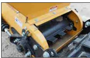
Fig 22 - Hopper end belt guard removed
