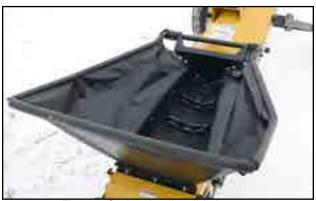
Fig 11 - Optional collapsible hopper
