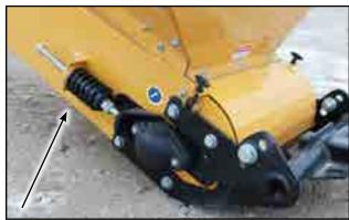
Fig 23 - Tension spring
