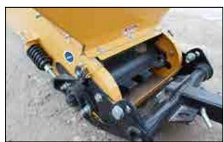
Fig 13 - Adjustable hitch. Belt guard is shown removed
