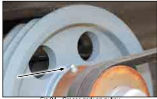
Fig 34 - Grease zerk on pulley
