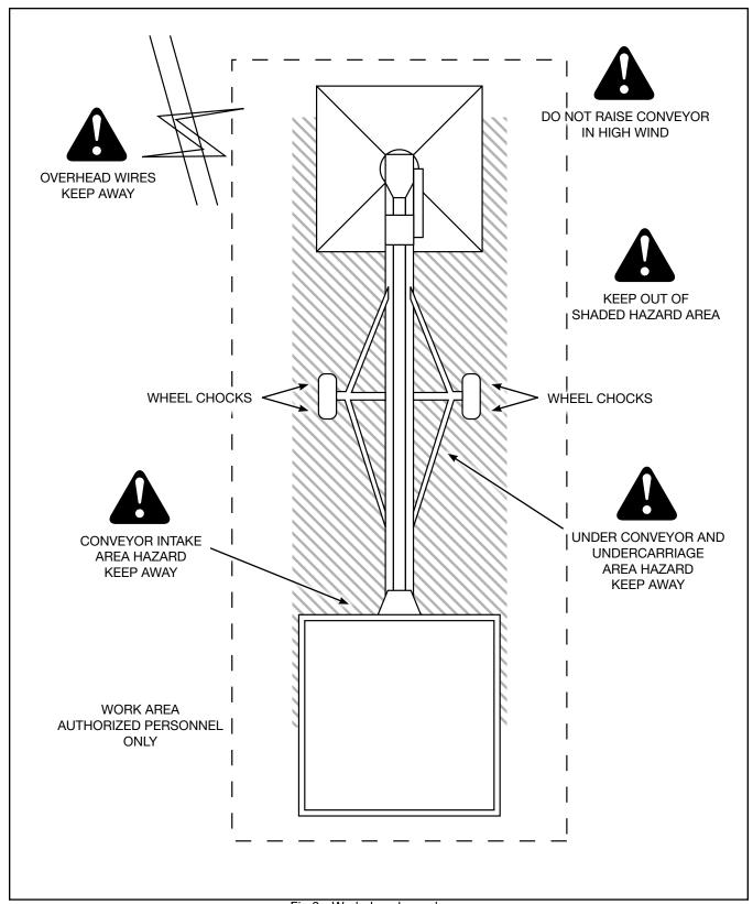
Fig 3 - Workplace hazard area
