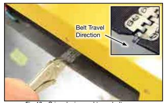
Fig 46 - Crimp lacing and taper belt corner
