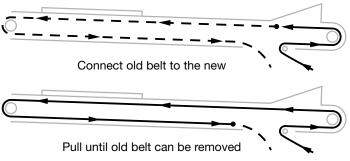
Fig 44 - Thread belt through conveyor
