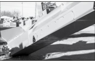
Fig 43 - Conveyor belt access panel
