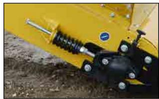
Fig 40 - Adjustment bolt and tension spring
