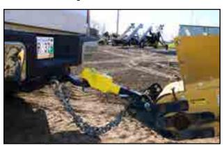
Fig 29 - Ball hitch with safety chains
