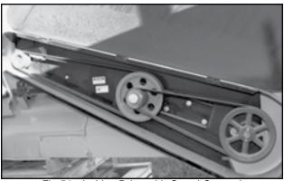
Fig 51 - In-Line Drive with Guard Opened
