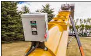
Fig 19 - Motor control box
