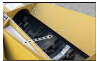
Fig 35 - Hopper flashing
