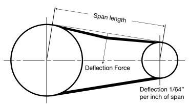
Fig 49 - Tension Calculation
