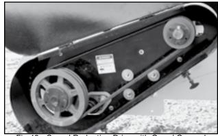
Fig 48 - Speed Reduction Drive with Guard Opened
